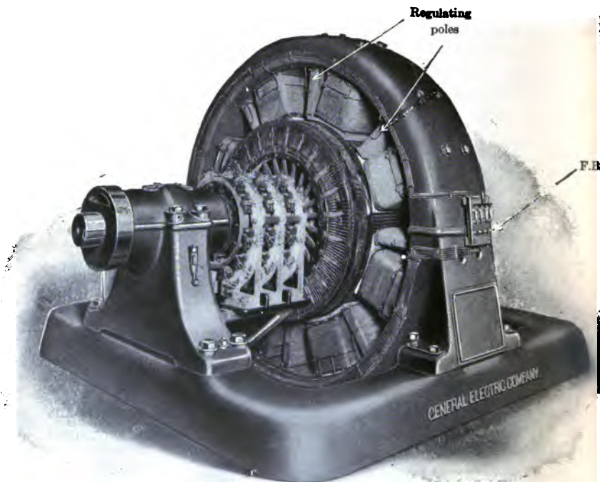
FIG. 328d. A regulating-pole converter. Note that each of the regulating poles is nearer one main pole than the other main pole.
